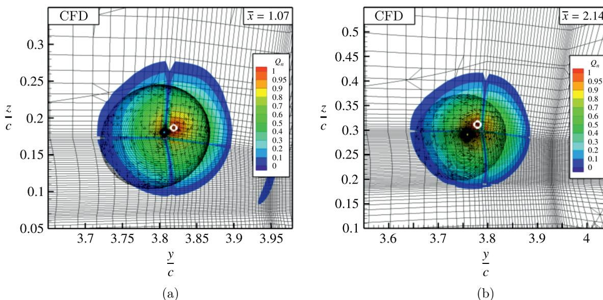
Figure 3. Location of the wing-tip vortex core centers using  $Q$ -distribution for various cross-sections: (a)  $\bar{x} = 1.07$ ; (b)  $\bar{x} = 2.14$
