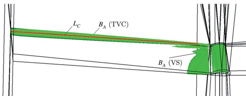
Figure 2. Visualization of the isosurface of the vortical core region  $W_A$  for  $\bar{Q} = 0.001$
