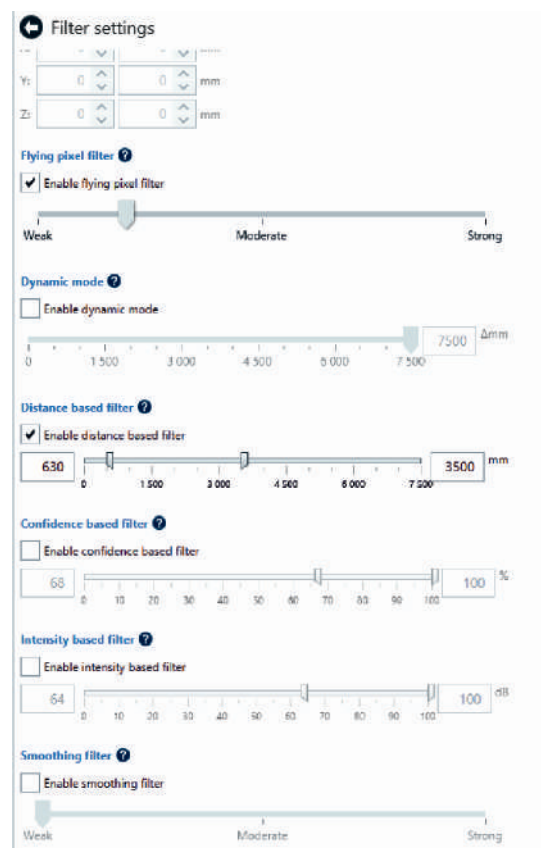
Fig. 2. Required parameters for adjusting the camera during the measurements: enable flying pixel filter — filtering of “floating” pixels — medium-weak; enable distance based filter — data filtering depending on the distance — no closer than 630 mm, no more than 3.5 m. We should also include other parameters, such as the dynamic mode, the confidence-based filter, the intensity-based filter, the smoothing filter
